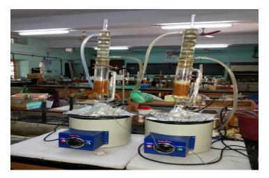
Fig.2. Soxhlet apparatus for the M.Tintoria roots extraction
